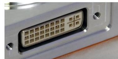
There are three types of DVI connectors based on the signals it can carry: DVI-I, DVI-D and DVI-A. DVI-I is a DVI port with integrated analogue and digital signals. DVI-D supports only digital signals and DVI-A supports only analogue signals.
