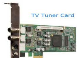
digital cable stations on the monitor. A TV tuner card can even provide a method for recording TV shows on the computer for later viewing, similar to how a Digital Video Recorder (DVR) device works. Internal TV tuner cards for desktop computers plug into either a PCI or PCI Express slot, and external TV tuners are also available for use with laptop and desktop computers. Some of these TV tuners also include a remote control for easy access and programming.
