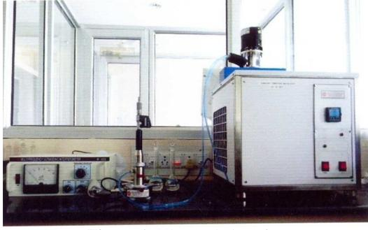
**Figure 1.** Ultrasonic interferometer
